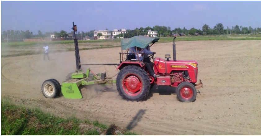
Fig. 11. Land leveling by laser land leveler
