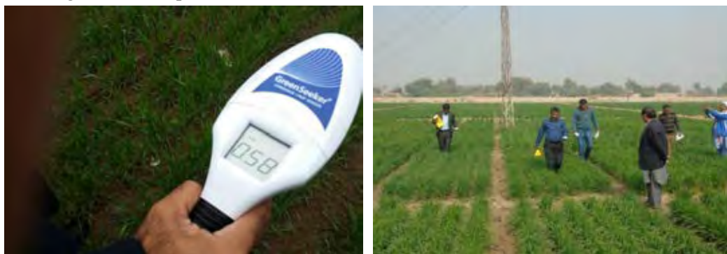
Fig. 19 Use of Green Seeker for wheat crop for nitrogen fertilizer assessment management
