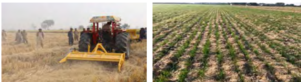
Fig. 13 Mulching of rice crop residues with residue mulcher before sowing of wheat crop
