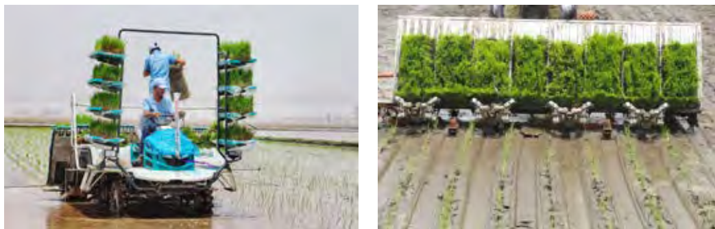
Fig. 9 Mechanical transplanting of rice
