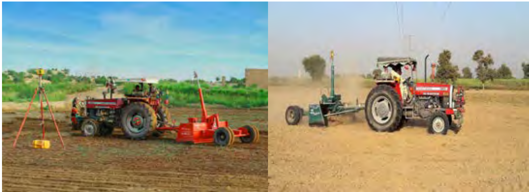
Fig. 3. Laser land leveling in the field
